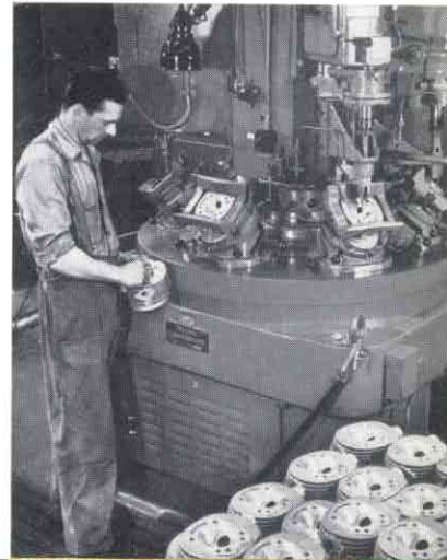
special boring machine for finishing cylinder heads
