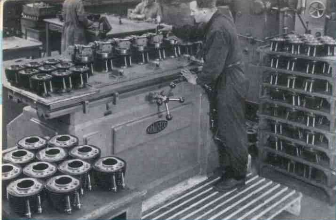
A special high precision cylinder boring machine.
