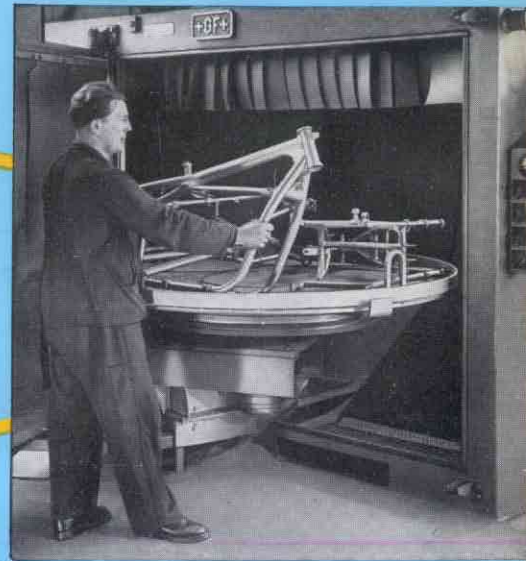
Modern sand blasting equipment, ensures a good paint finish.
