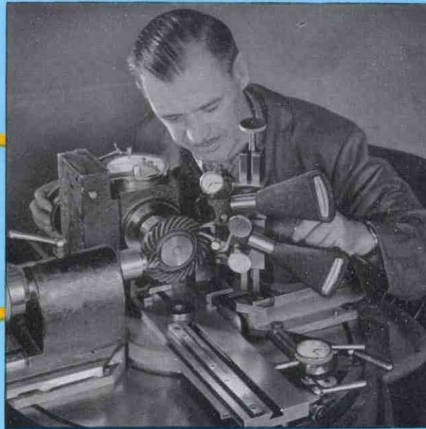
Rear wheel drive bevel gears are inspected with special gauges.
