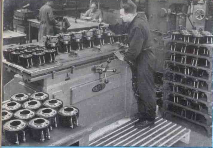
A special high precision cylinder boring machine.
