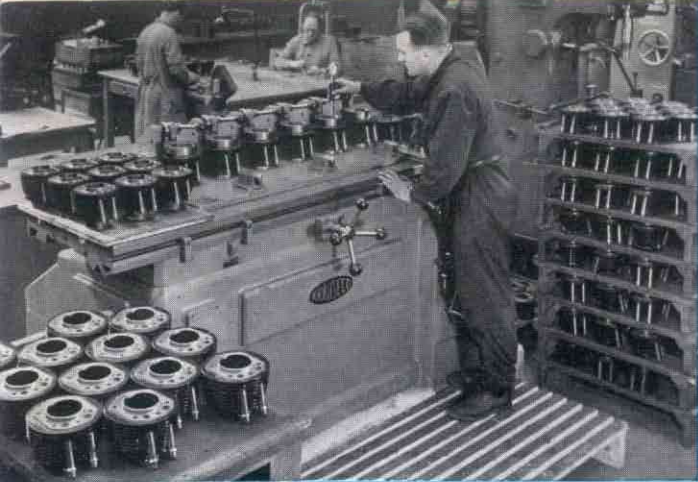
A special high precision cylinder boring machine.
