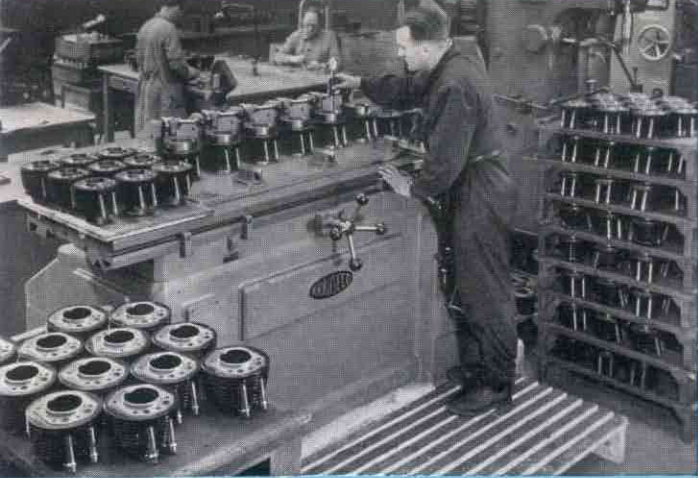
A special high precision cylinder boring machine.
