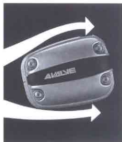
Ideal thermal balance. Protruding to the side, both cylinders are cooled perfectly by the wind rushing by. They also help protect the rider in the event of a fall or side collision.
