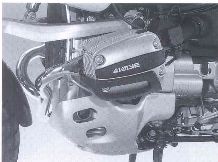
When the going gets tough, the new BMW GS has all the necessary fittings as standard. For example, undertray and cylinder guards.
