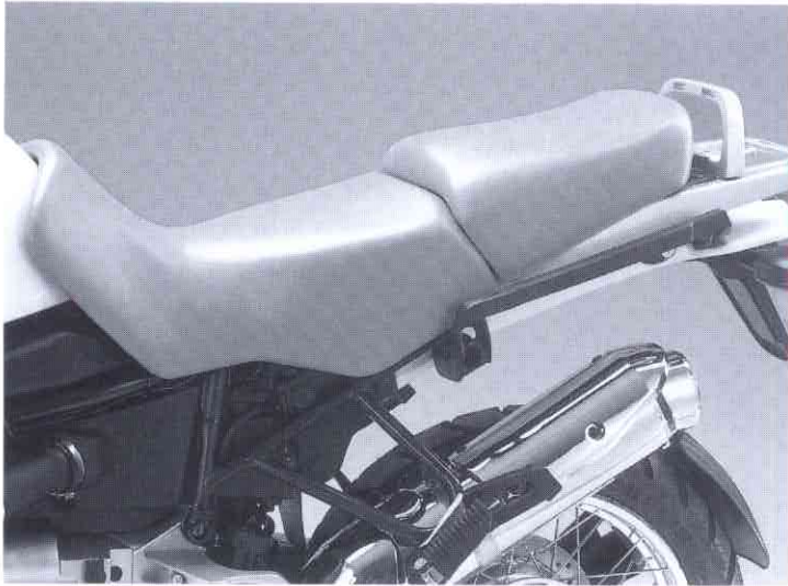
Now adjustable: the rider can choose a seat height of 33.6 or 34.4 inches.
