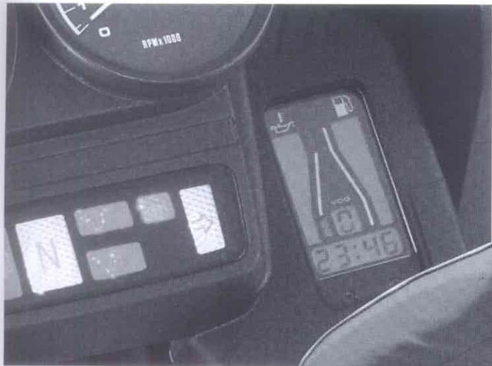
The rider information display (optional extra) shows the time, gear currently selected, fuel level and oil temperature at a glance.
