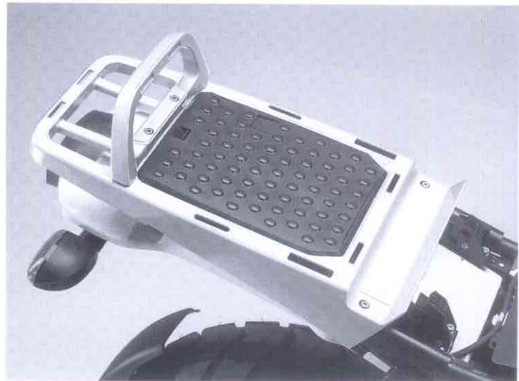
Perfect for long-distance riders: the luggage rack beneath the detachable pillion passenger's seat can be used to secure a large number of articles. This ideal arrangement keeps the motorcycle's center of gravity low.
