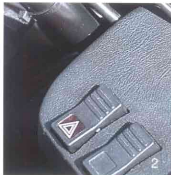
2 Safety first: BMW hazard warning flashers can be retrofitted easily on all BMW machines.
