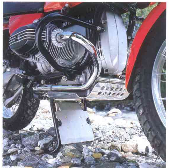
6 The BMW touring case comes in asymmetric design to fit the high rising exhaust pipe on the BMW enduro. And there's a special top case to match; the extra-sturdy leather bag mounted on the rear.
