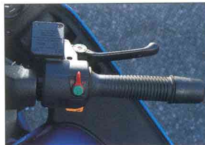
Softer grips, bar-end weights to damp out vibration and a thumbwheel adjuster on the brake lever are new for '93.
