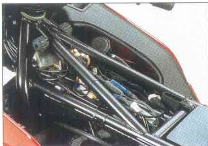
K1100RS frame rigidity is enhanced by a pair of backbone struts in place of the single strut in last year's frame.
