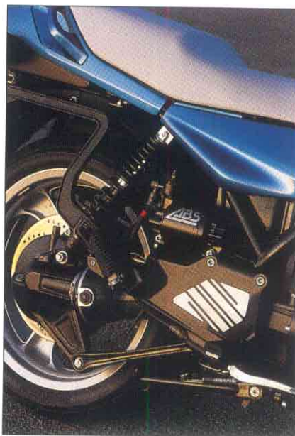
Footpeg mounting system is vibration isolated from frame and engine. BMW by Showa shock has progressively wound spring, adjustable rebound damping.
