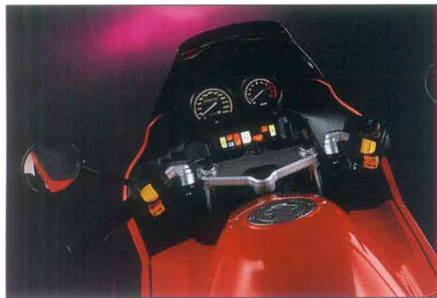
Simple, readable instrumentation and BMW's now-familiar hand controls. Also visible on the right side of the dash is the optional instrument pod that gives time, oil temperature, fuel level and gear selected.
