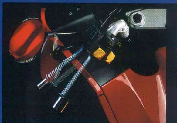
BMW's second-generation ABS does away with the unattractive, heavy and hard-to-hide twin solenoids of the original ABS set-up. The new system's motor is hidden under the fuel tank.
