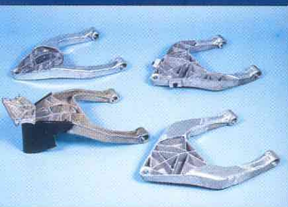
Various versions of the front A-arm. When aluminum arms did not deform sufficiently in crash tests, steel arms were fitted.
