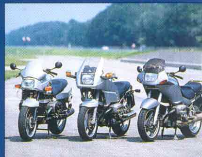
R1100RS prototypes. From left to right, the 1989 version, the 1988 version (with K100 fairing) and the 1990-91 version.
