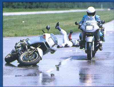
Panic-brake testing on a wet surface. Guess which RS prototype is equipped with anti-lock brakes.
