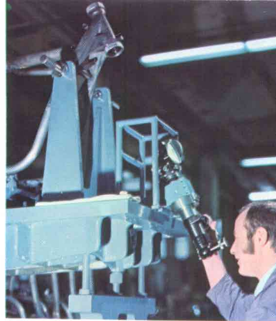
Optical sighting rig checks alignment of steering head and frame tubes.
