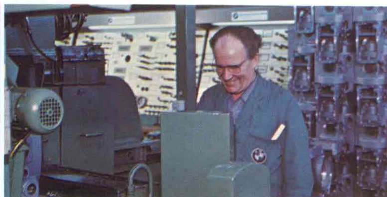
Crankshaft runout readings are displayed and recorded. Vast control board at rear signals any tolerance error.
