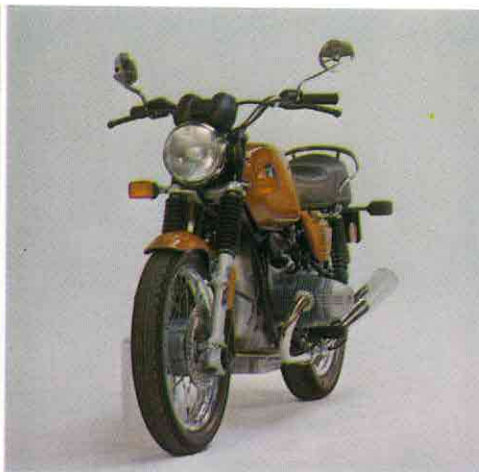
Among many new features: safety gas caps, standard 6.3 gallon tanks, perforated disc brakes, and redesigned valve covers.
