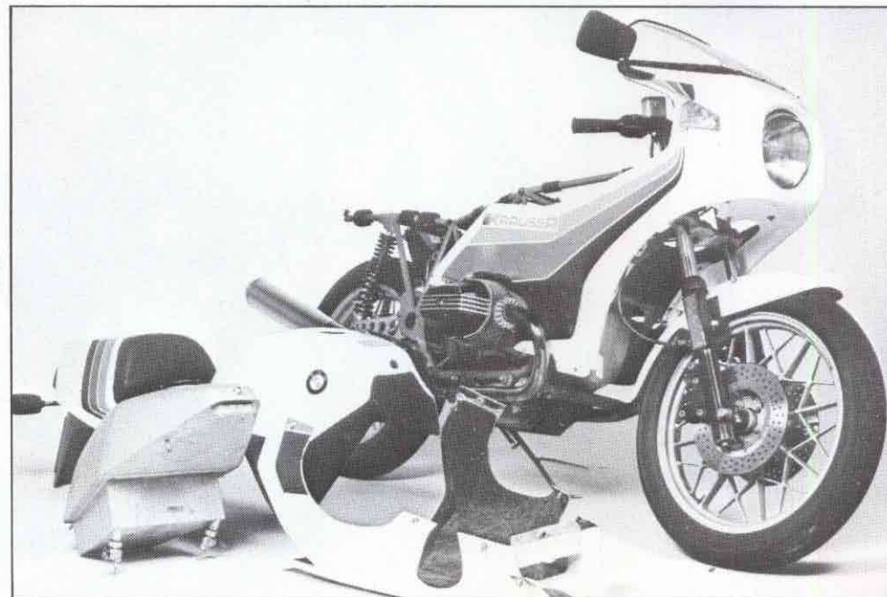
Above: the 21 litre alloy tank sits neatly in the frame, but the taps caused problems. Top right: light, low, strong, the Krauser frame is an unlikely but noticeable improvement. Below: the rest of the kit is high quality and fits well.
