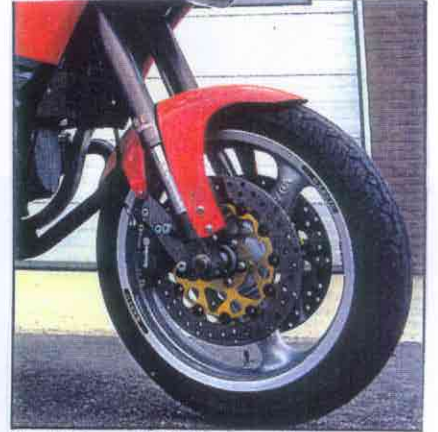
Front forks are White Power upside-downies, brakes are 300mm Brembos with four-piston callipers. No problems tying your Kangaroo down
