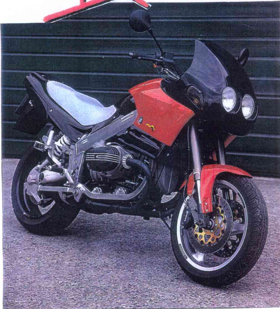
Front forks are White Power upside-downies, brakes are 300mm Brembos with four-piston callipers. No problems tying your Kangaroo down
