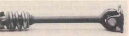
The RT's all-new shock-equipped driveshaft cushions rear end and gearbox, and helps gear disengagement.
