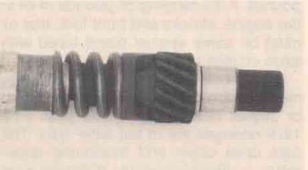
Power from the clutch is transmitted to the gearbox with this shock-absorber-equipped input shaft.
