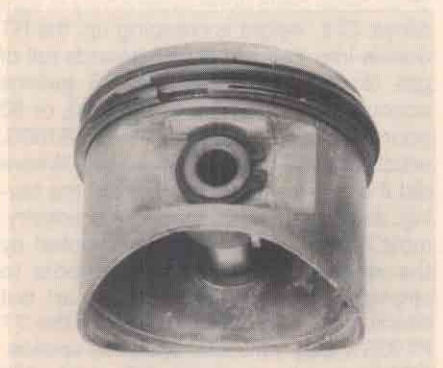
Beemer pistons, made either by Mahle or Kolben Schmidt, use external pin retainers and three rings.
