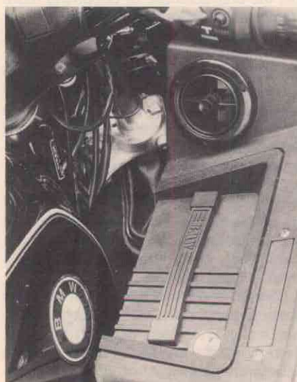
"Oddments compartment" holds about six liters and needs a hinge. Air vent closes with a butterfly valve.
