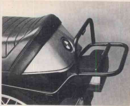
Integrated saddlebag mount and rack provide little load capacity without bags; tail lamp uses two bulbs.
