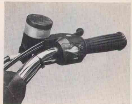
Due to beneath-the-tank space requirements, BMW moved the front brake reservoir atop the handlebar.
