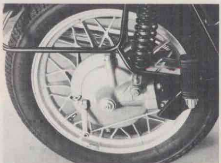
Ordinary rear brake, unique final drive ratio. The R65 has low 3.44:1 gears to help out smaller engine.
