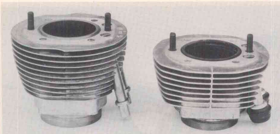
R65 (right) and R100 cylinders illustrate dramatic "width" difference accounting for much narrower engine.
