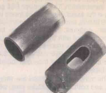
Valve lifter from the 650 (above) is hollow, allows long pushrod length to be maintained.
