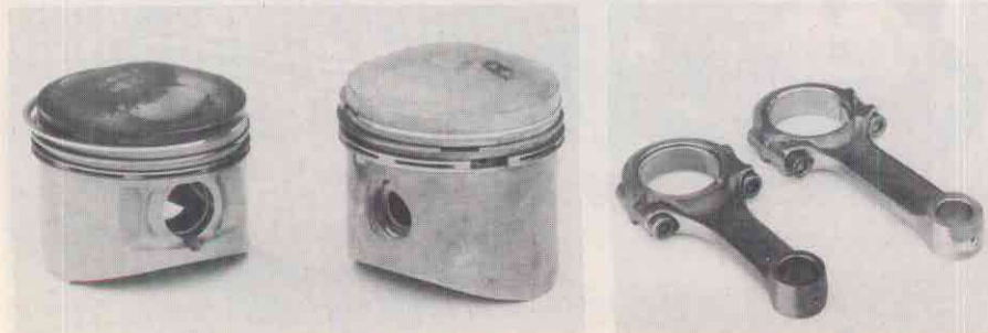
More subtle size differences are apparent in pistons . . . . . and forged steel connecting rods.
