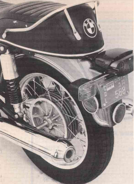
Spider hub-design uses straight-pull spokes which are stronger than ones which bend at the flange.
