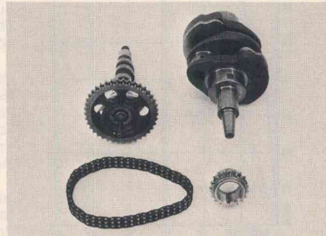
Camshaft drive by automatically tensioned duplex chain comes straight out of BMW's rally-winning sports sedans. Valve timing affords a generous 88 degrees of overlap, which makes for good combustion chamber filling, easier starting, higher midrange torque.
