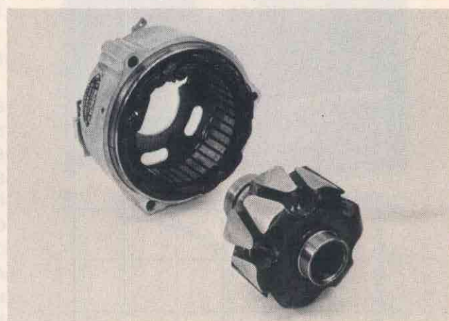
Three-phase 180-watt alternator gets magnetization current for rotor from the battery. Alternator has advantages of compactness, efficiency, and no rubbing connections (brushes) for high currents. The alternator output will fire plugs—even if battery fades to seven volts.
