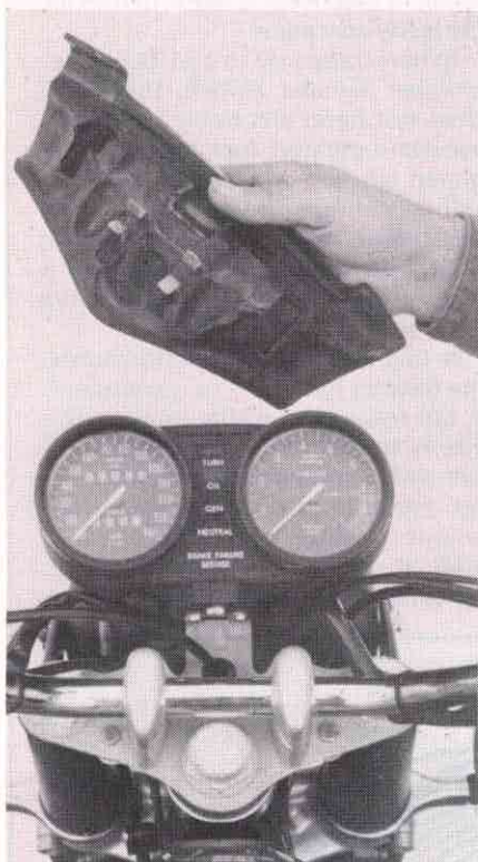
The "padded dash" fitted to all '78 BMWs may be snapped off and discarded if the owner doesn't like it—or if a passerby does like it.
