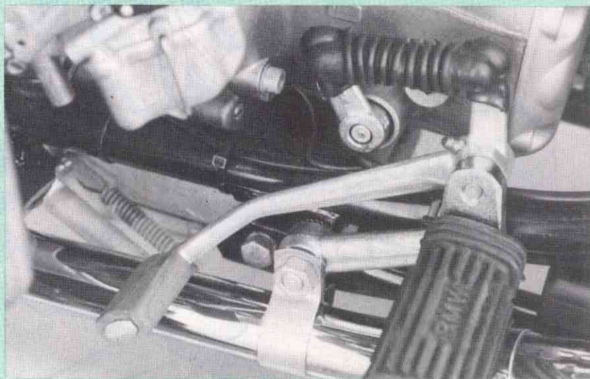
The new shift linkage results in more positive gear-changes because the new pivot point provides more leverage.
