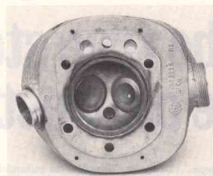
Slash-Six series is highly rationalized; R75/6 head caps an 82mm bore rather than 90mm hole.
