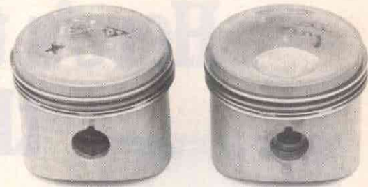
R90/6 piston on left is 9.0:1; higher compression R90S piston has larger dome.
