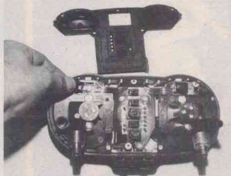
Back side of instrument panel shows easy to replace lamps and a printed circuit board instead of wires.
