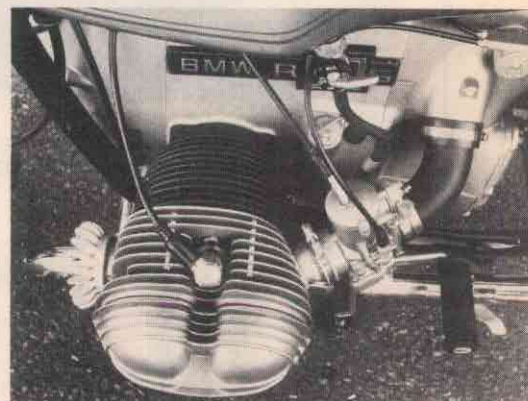
BMW's opposed-twin engine layout, with air-cooled cylinders and air-warmed toes.
