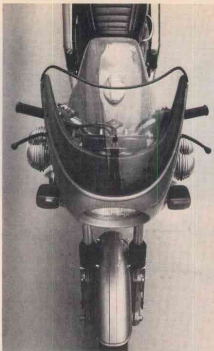
The abbreviated fairing isn't streamlining; it deflects the wind from the rider's body.
