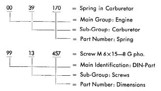
When looking for a part number (ordering number) of a part, find the figure call-out number in the illustration of the main group, and find the part number in the associated text which corresponds to the call-out number. When ordering parts it is advisable to specify the frame and engine serial numbers. Parts for which no figure call-out number exists will be found listed in the text under the group to which they belong.
