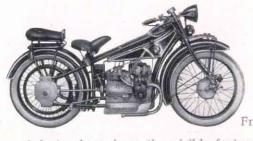
From the very beginning, particularities of design have been the visible features of BMW motorcycles. Already on the first BMW motorcycle which was built in 1923 the reliable opposite-twin engine with shaft drive served as source of power. This design which aroused great interest has been developed step by step up to its technically mature shape of to-day. The high quality of BMW motorcycles has established their excellent reputation — riding them proves their value.
