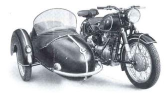
R 26 with BMW "Standard" sidecar. Swinging axle and body equipped with rubber springing. Hydraulic braked sidecar wheel. Four-point ball joint attachment. Carries three people.
