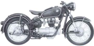
Powerful single cylinder engine. Special large air-intake ensuring cool and uniform air supply. Four speed gearbox with foot change. Very elastic clutch. Front and rear wheel suspension with suspension units and double
