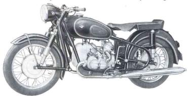
with racing motorcycles. Polished 18 in. light-alloy wheelrims. Full-width hubs with large diameter brakes. Stop light. Sprung sports seat or pillion seat.
