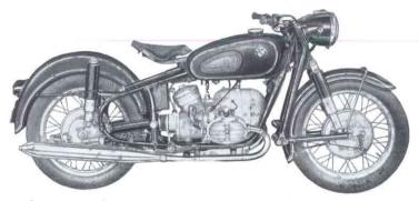
racing motorcycles. Polished 18 in. light-alloy wheelrims. Fullwidth hubs with large diameter brakes. Stop light.
