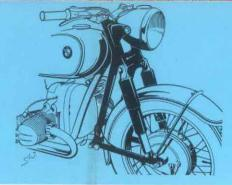
R 50 TOURING-SPORT 500 c. c. 26 hp. Powerful two cylinder engine. Hydraulic damped swing frame with suspension units and hydraulic shock absorbers based on experiences gathered with
