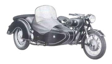
Sidecar swinging axle and body equipped with rubber springing. Oil pressure braked sidecar wheel, available also for solo use.
