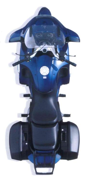
Two-cylinder Boxer engine with 4 valves per cylinder Displacement: 1085 cm<sup>o</sup> Output: 66 kW (90 hp) at 7250 rpm Torque: 95 Nm at 5500 rpm Mixture control: Basch Matronic MA 2.2 with overrun fuel cutoff: closed-loop 3-way catalytic converter (optional)
