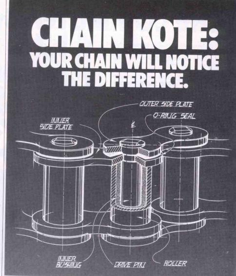
Kal-Gard Chain Kote provides each part of your chain with the lubrication it needs to run smoothly and quietly, and last a long time. A clear understanding of your chain will help you realize that it requires sophisticated lubrication in order to take what your engine dishes out.
