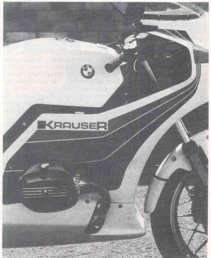
All glass fibre-work is manufactured under the machine sprayed chopped fibre and resin mix method. The finish was at least as good as an RS's fairing, but to a much lighter standard, although the fairing was stiff and its mounting rigid
