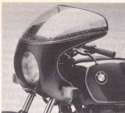
The R100S nose fairing keeps the airstream off the rider's torso and provides coverage for the instruments.
