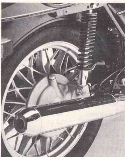
Handle, not tool-kit tool, adjusts shock-spring preload. Disc holes improve BMW's wet-weather braking.
