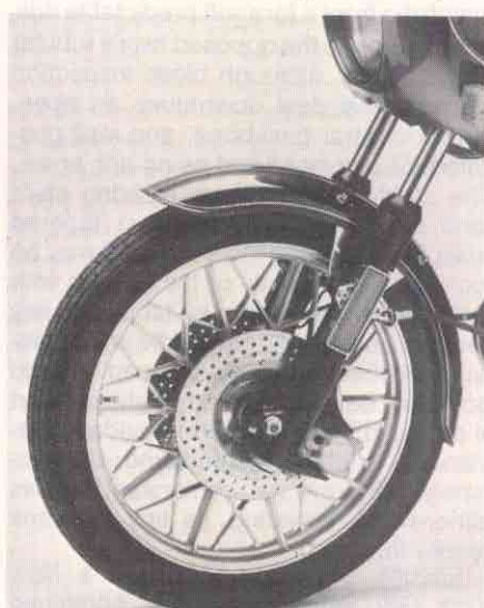
Handle, not tool-kit tool, adjusts shock-spring preload. Disc holes improve BMW's wet-weather braking.
