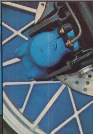
The optional aluminum wheels are slightly heavier than wire ones, but help handling.
