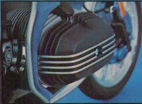
New rocker covers are black-anodized with polished fins; they're a little bigger, a bit heavier and great-looking.
