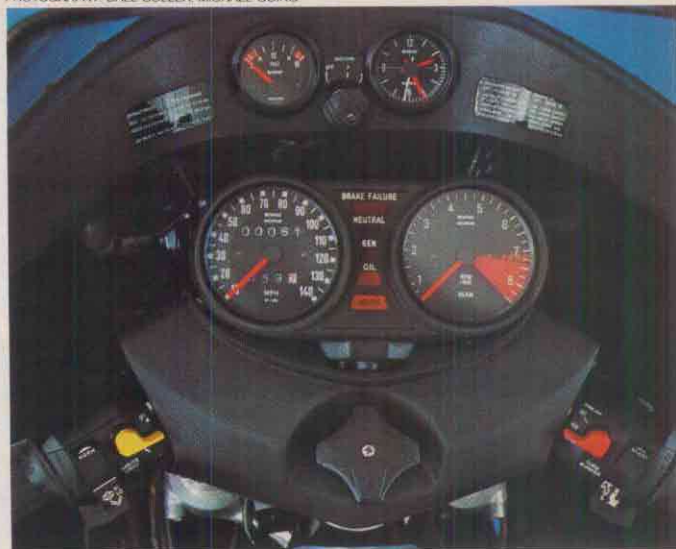
Like the R90S, the R100RS comes with complete instrumentation: voltmeter, speedo and tach, clock, and warning lights galore. Wanna take your own lap times?
