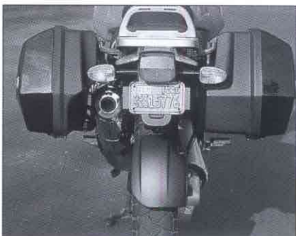
Tough, easily operated saddlebags are a worthy option, but accommodating the upswept muffler robbed the left one of some volume.
