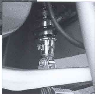
Above: The shock in the Telelever front end is adjustable for spring preload. Middle right: Pulling the rear seat reveals a large platform for luggage which is also the lockable lid of the well-equipped tool case.
