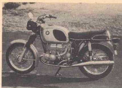
All fenders are now made of fiberglass to lighten the load for the 600cc mill.
