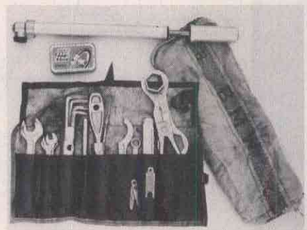
The tool kit is excellent. The 25-piece kit includes tire irons, a pump, a tube patch kit, and a monogrammed polishing cloth.
